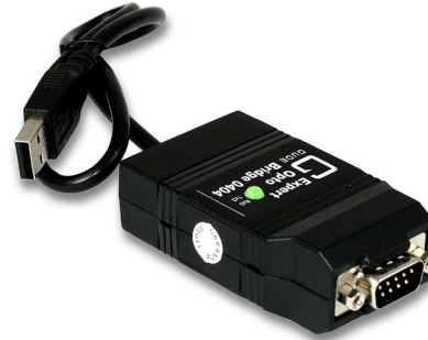
Expert Opto Bridge 0404: USB-/RS232 converter with galvanic interface isolation
