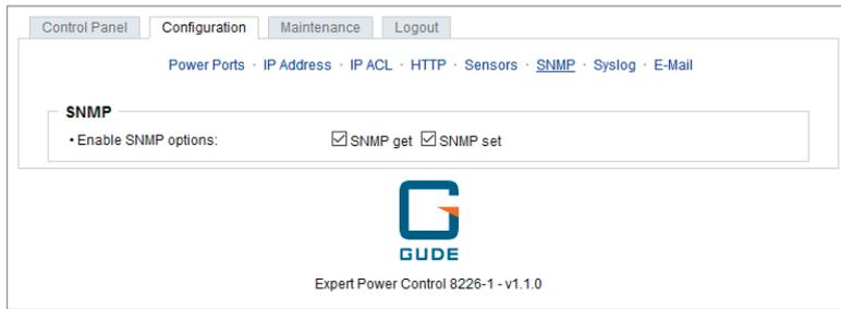
Fig. 5: Activating SNMP in device's web interface
